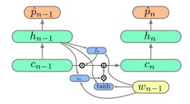
$$\begin{split} i_n &= \sigma \left( W_i[w_{n-1}; h_{t-1}] + b_i \right), \\ f_n &= \sigma \left( W_f[w_{n-1}; h_{t-1}] + b_f \right). \end{split}$$
