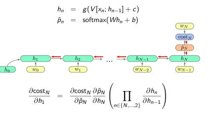
$$h_n = g(V[x_n; h_{n-1}] + c), \qquad \frac{\partial \operatorname{cost}_N}{\partial h_1} = \frac{\partial \operatorname{cost}_N}{\partial \hat{\rho}_N} \frac{\partial \hat{\rho}_N}{\partial h_N} \left( \prod_{n \in \{N, \dots, 2\}} \frac{\partial h_n}{\partial h_{n-1}} \right)$$
