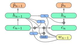
$$i_{n} = \sigma (W_{i}[w_{n-1}; h_{t-1}] + b_{i}),$$
